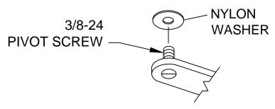
1000T, 1000SLT, 9000T 9000AT REPLACES THE JAMB BRACKET WITH A THREADED NYLOK JAMB PIVOT SCREW
