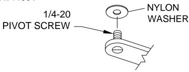
3300AT, 4000T & 4400T REPLACES THE JAMB BRACKET WITH A THREADED NYLOK JAMB PIVOT SCREW
